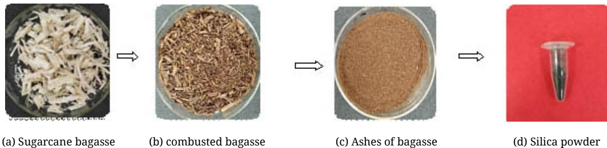
Fig. 1. Synthesis of silicon nanoparticles from agro-waste (Sugarcane bagasse)
