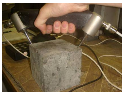
Fig. 4. Ultrasonic pulse velocity method
