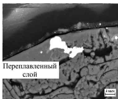
Fig. 11. Scanning electronic microscope image of coating cross-section: а – prior to exposure to compression plasma flows; б – the same after exposure
