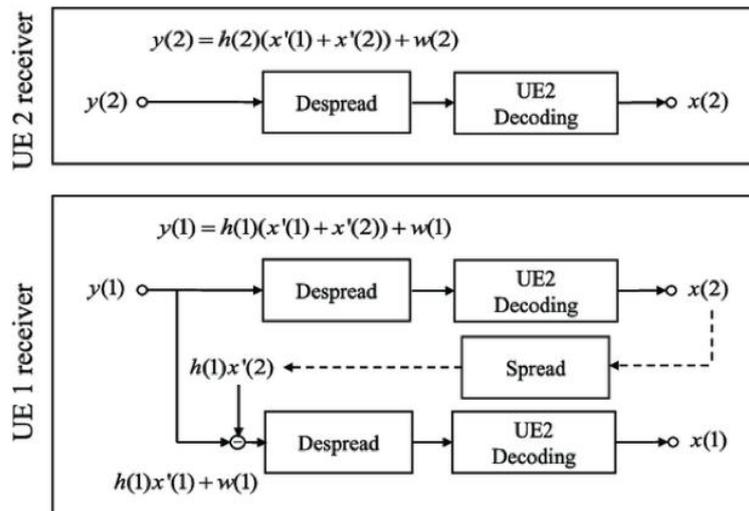
Fig. 4. The process of signal detection by user UE  $I$
