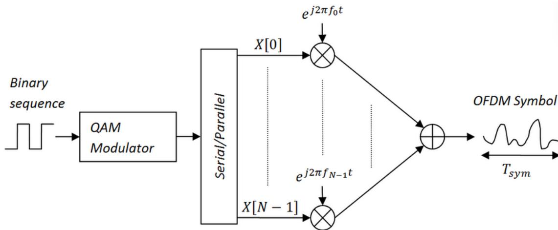
Fig. 1. The model of modulation in OFDMA
