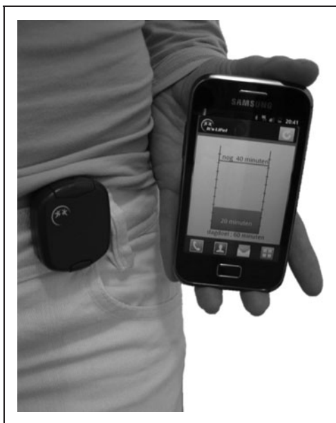
Fig. 1. The It's LiFe! monitoring and feedback tool. The MOX and the real-time feedback (activity results in minutes a day compared with a personal goal) on the smartphone application are shown.
