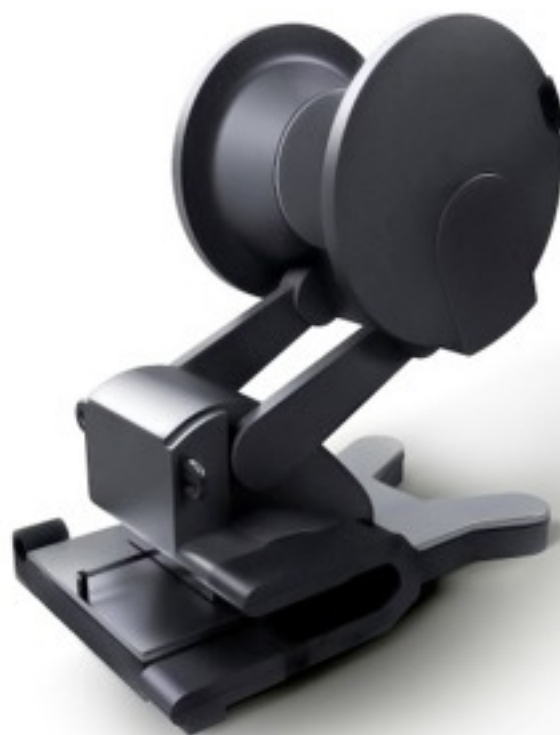
Figure 1.1: PoleStar N20 (0.15 Tesla) intraoperative MRI
