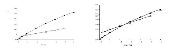
**Figure 3**. TEB conversion as a function of time: ( $\square$ ) ambient pressure ethanolysis reaction; ( $\square$ ) ethanolysis reaction in CO<sub>2</sub>-expanded media. Solid lines: values calculated using Eq. (2).
