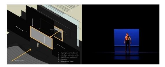
Caption: The three automated curtains moved vertically and horizontally allowing dynamic framing of action on the stage.
