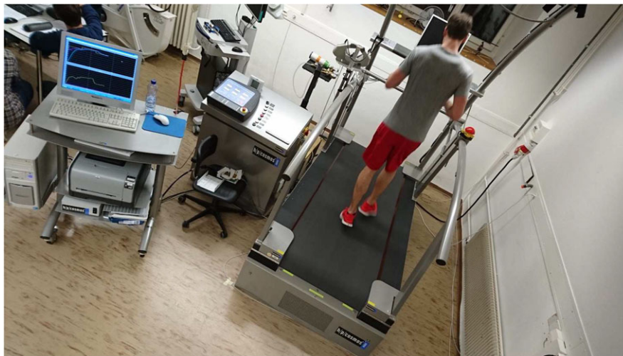
FIGURE 3 Computer-controlled treadmill. Controllers were implemented in real time in the PC on the left. The control signal (speed command) was sent via serial link to the treadmill control unit in the centre [Colour figure can be viewed at wileyonlinelibrary.com ]
