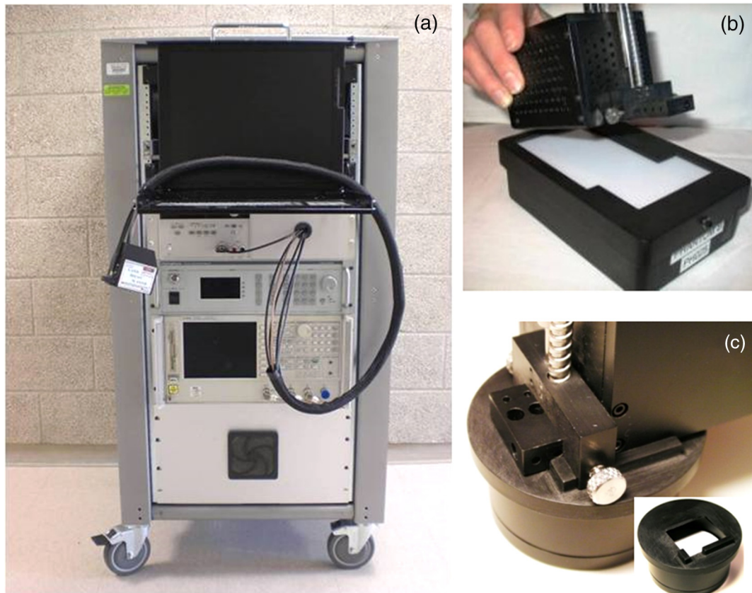
Fig. 1 (a) DOSI instrument and (b) and (c) illustrate the probe placed on the calibration phantom (FDPM calibration) and on the reflectance standard (broadband calibration), respectively.
