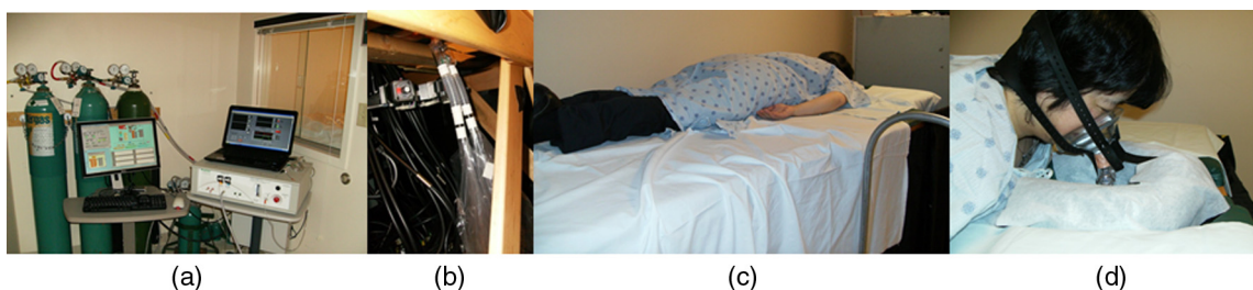
Fig. 2 Views of the imaging room. (a) Console area for NIRS and gas supply control system (Respiract™). Exam table is located behind the window. (b) The breathing circuit under the table next to the fiber optical interface. (c) A subject lying prone on the breast exam table. (d) A subject with facemask before being positioned on the headrest.
