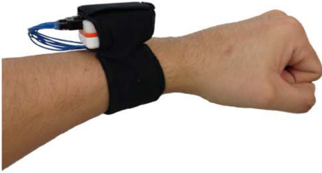
Figure 1: A subject wearing one of our bioimpedance sensors. The exposed wires connect the electrodes to our custom sensor module (which is connected to the Shimmer via the internal expansion port).
