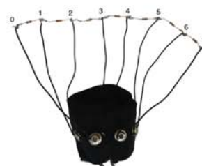
Figure 15: The resistor array used to calibrate our system. The 1\text{ k}\Omega \pm 5\% resistors are connected in series. The reference resistance between a pair of electrodes will vary depending on the number of resistors between them. For example, the resistance between electrodes 0 4 is 4\text{ k}\Omega .
