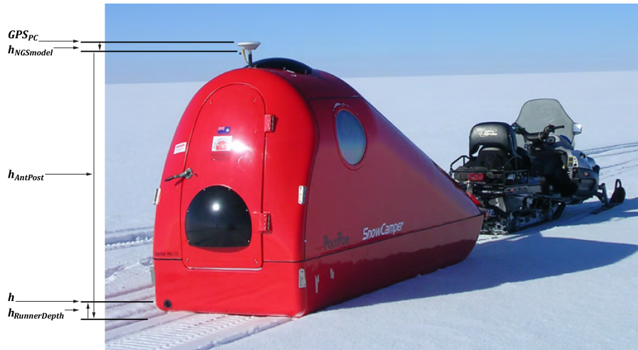
Figure 2. The roving GPS antenna, sled, and snowmobile configuration. GPS_{PC} is the surveyed position solution to the phase center of the antenna, h_{NGSmodel} is the NGS model distance between the antenna phase center and the antenna base plane, h_{AntPost} is the height of the antenna post (Table 1), h_{RunnerDepth} is the depth of the sled runners in the snow surface (Table 1), and h is the snow surface (Eq. 1).
