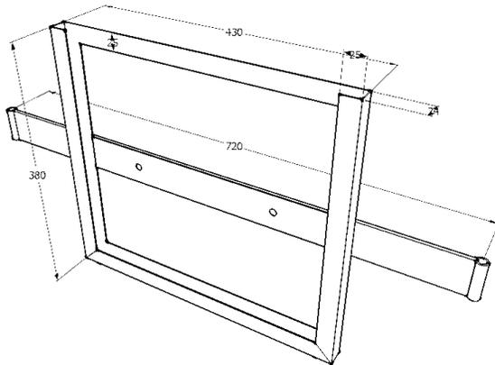
Gambar 5.a. Rangka Flat Panel
