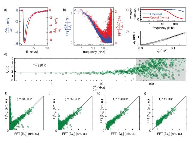
OLED operating with a constant forward bias of 4 V. (a) Plots of the relative current changes  $\delta J_{\rm E}/J_{\rm E}$  as well as the relative change of the detected EL intensity  $\delta J_{\rm V}/J_{\rm V}$  following a short
