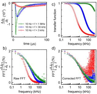
PPV OLED. A constant forward bias of 3.73 Volts was applied to the device. (a) Plots of the relative current changes  $\delta I_E/I_E$  follow a short microwave pulse of duration 400 ns and frequency 9.625 GHz, as a function of time after the pulse for three different band-pass
