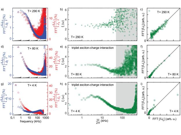
FIG. 5. Simultaneous room-temperature measurements of pEDMR and pODMR on a SY-PPV OLED at various temperatures. (a) Plot of the magnitude of the FFT of the transient relative current change  $\delta I_E/J_E$  as well as the transient relative change of EL  $\delta I_\gamma/J_\gamma$ following a short microwave pulse of duration 400 ns (frequency 9.6240 GHz). A constant forward bias is set to V = 13.7 V at T = 100 K. (b) Plot of the ratio
