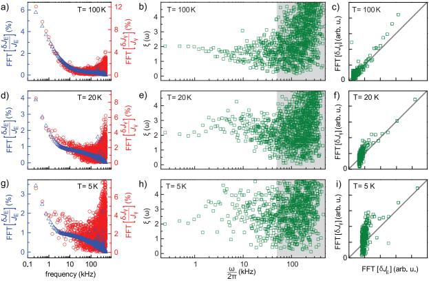
PPV OLED at various temperatures. (a) Plot of the magnitude of the FFT of the transient relative current change  $\delta J_{\scriptscriptstyle E}/J_{\scriptscriptstyle E}$  as well as the transient relative change of EL  $\delta J_{\scriptscriptstyle \gamma}/J_{\scriptscriptstyle \gamma}$ following a short microwave pulse of duration 400 ns (frequency 9.6232 GHz). The constant
