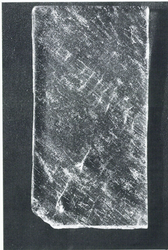
Fig. 2. Photograph showing across-column cracks in a specimen shortened 0.2% at 1 \times 10^{-4} \text{ s}^{-1} . The load was applied in the vertical direction. Note the sets of cracks which appear to have traversed a grain and to have initiated and terminated at the boundaries. Scale: specimen width = 50 mm.
