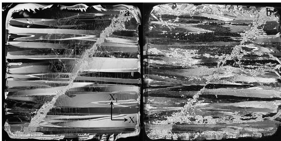
Fig. 1. Photographs of a P-fault in thin sections of (a) columnar freshwater ice and (b) columnar saltwater ice as viewed under polarized illumination. Faulting generated under (1.0:R_{21}:R_{31})=(1.0:0.5:0.2) at T=-20^{\circ}\text{C} at \dot{\epsilon}_{11}=1\times 10^{-1}\text{s}^{-1} . Minimum feature size on scale is 1 mm.
