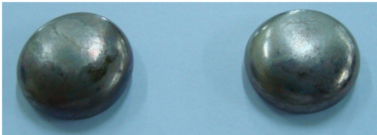
Gambar 3. Ingot paduan U-Mo hasil peleburan
