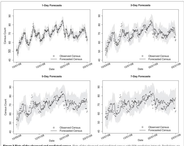
**Figure 3 Plots of the observed and predicted census.** Plots of the observed and predicted census with 95% prediction intervals. Predictions are based on data observed up to the date being predicted.
