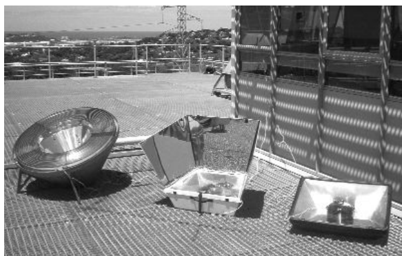
Figure 3: Clear-sky performance tests, with (left to right) the RACStove and ovens C1 and C2
