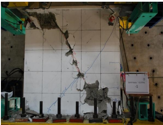
Figure 4.4.a Crack of position at drift ratio 0.35%, experimental wall
