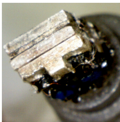
Figure 2. Top view of temperature regulated platform, and Ag sample thermometer/spacer, and heater frames.
