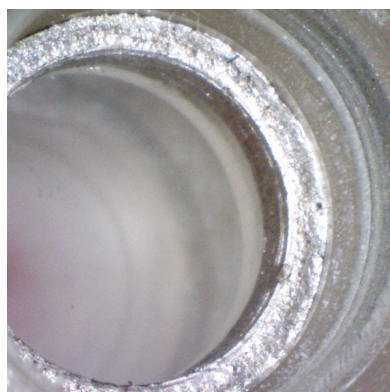
Figure 1. PDF calorimeter cap interior, showing sample chamber, step edge, indium gasket, and internal threads.
