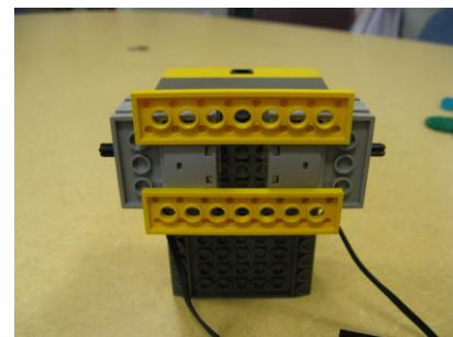
(c) Reinforcement of motors
