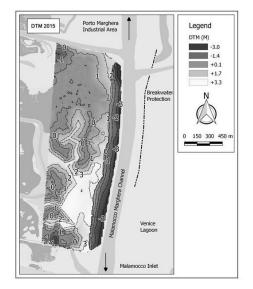
Fig. 2. Digital terrain model (DTM) of the studied area. In dark gray (negative values) the volumes removed from 1970 and 2015.
