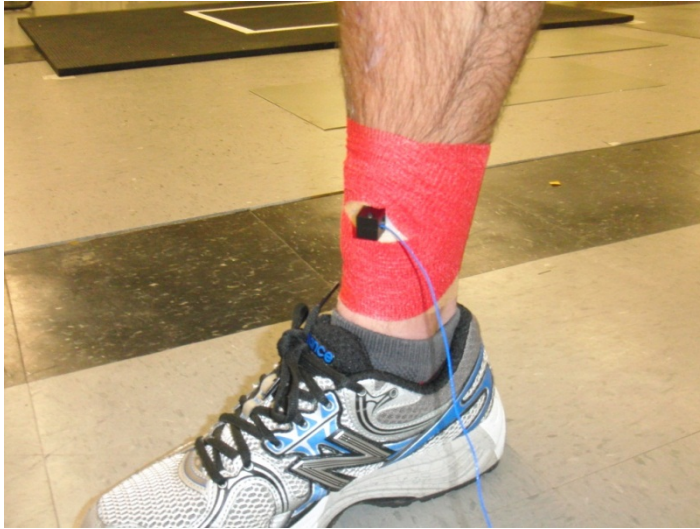
Figure 3.1- A uniaxial accelerometer, housed in a custom chamber and mounted to a moldable plastic cuff, was attached to the distal, anterior tibia with pre-wrap tape.
