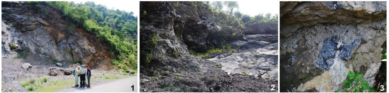
Fig.4. 12 Field photos at LS1. 1 in Fig. 4. , Steep and strongly sheared Paleozoic sedimentary rock. 2, A boundary of the landslide body and the slip surface. 3, Close up the boundary.
