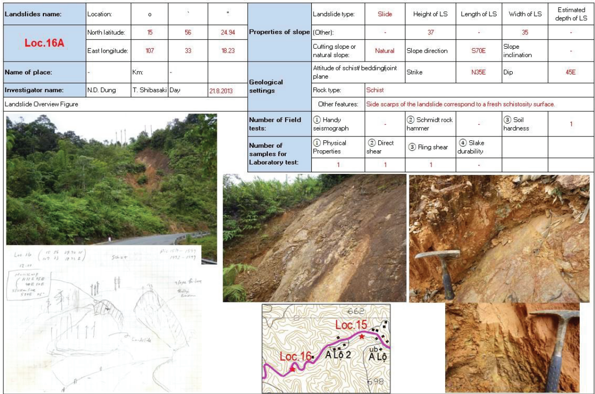
Fig.4. 48 The Landslide field Inspection sheet of Loc.16A
