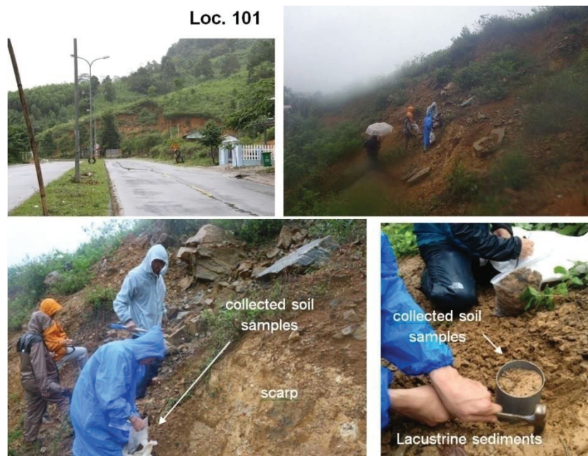
Fig.4. 24 Collected soil samples at landslide Loc.101 on HCMR around KhamDuc area
