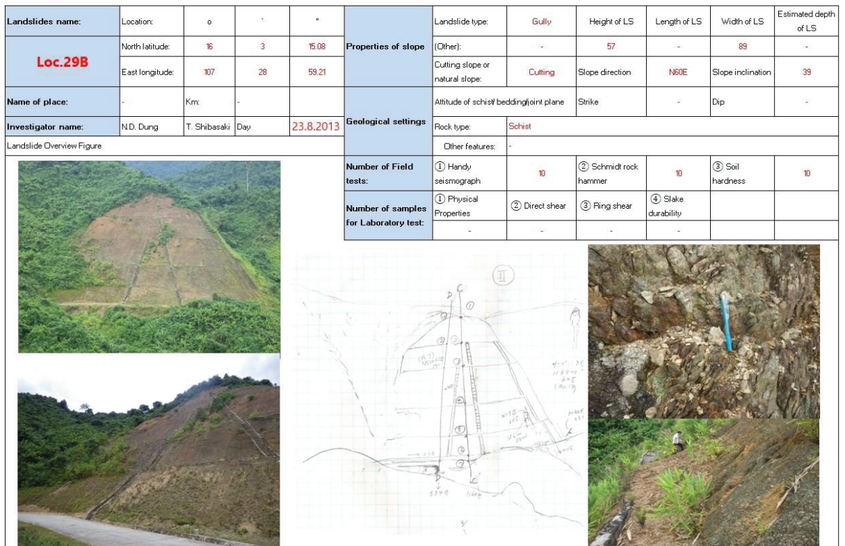
Fig.4. 63 The Landslide field Inspection sheet of Loc.29B
