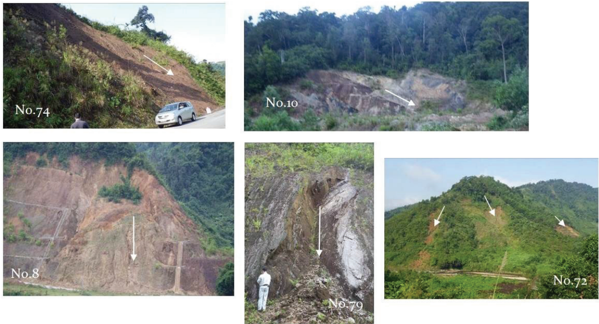
Fig.4. 19 Moving types of landslides along HCMR (No74: Translational shallow debris slide, No.10: Translational rock slide, No8: Rotational slide, No.79: Translational wedge type slide, No.72: Gully type slide and flow) (Abe et al., 2014)
