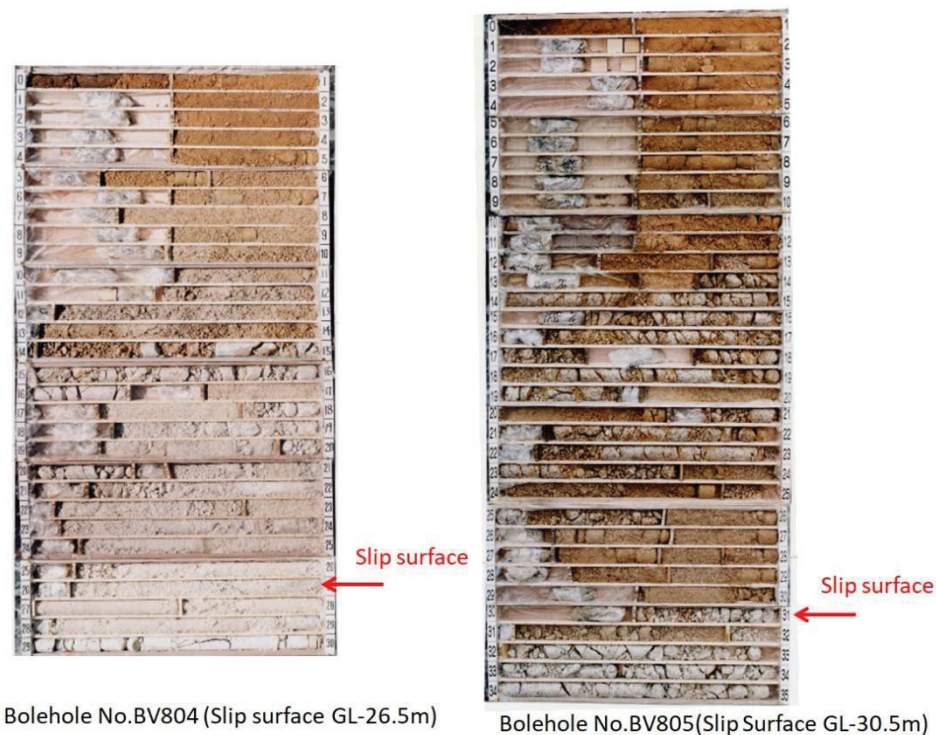
Fig. 3. 9 An example of geological drilling for identifying slip surface of landslides in Japan
