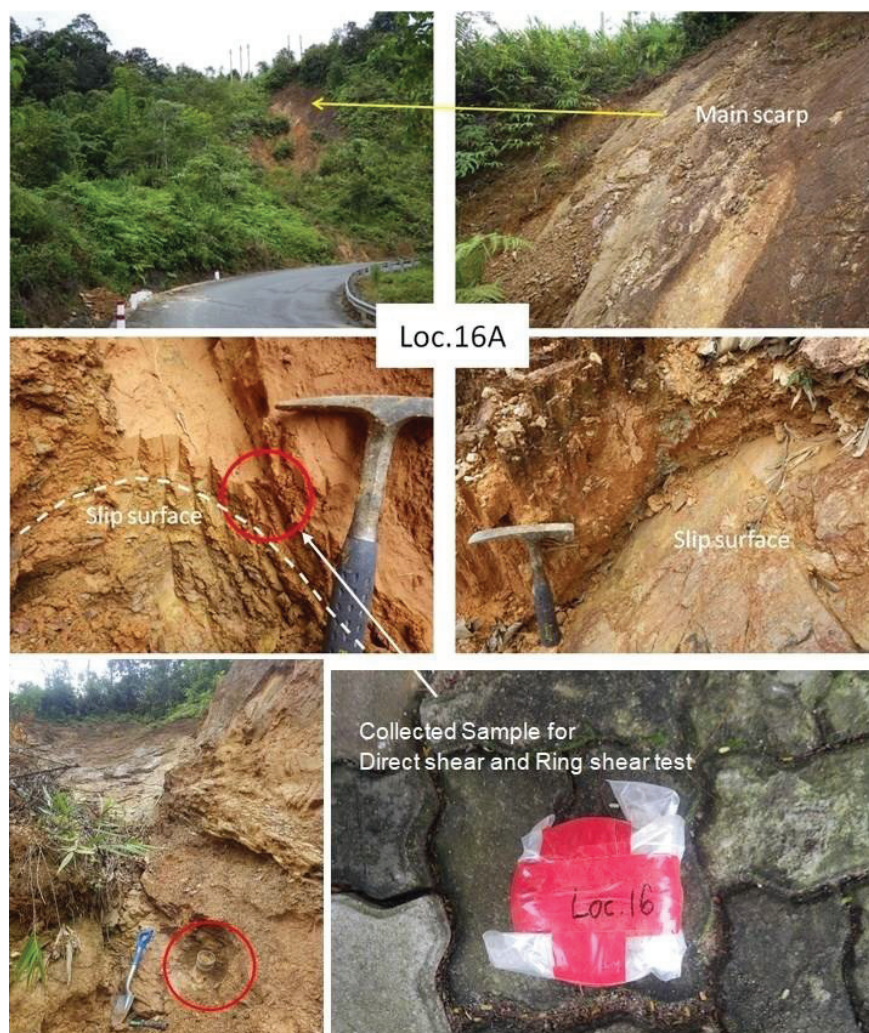
Fig.4. 23 Identified slip surface at the field and collected soil samples at landslide Loc.16A
