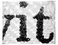
Figure 5 Photomicrograph of gravure printing. Note uniform irregularity of edges
