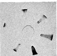
Figure 2 Horizontal Chromatograms of Typical Ball Point Inks
