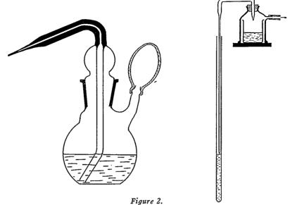
Left: Micro Wash bottle, 50 ml., for charging gradient tubes. Right: Suction device for adjusting liquid levels.
