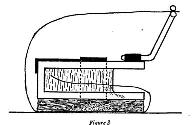
Arrangement for Collecting Blood from Vertical Surface. Metal frame and suction cups indicated.
