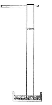
Figure 1 Simple arrangement for collecting blood from debris by filterpaper.
