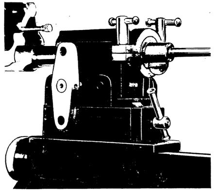
FIGURE III Rifling meter head stock with barrel in place and supplementary clamp referred to in text.
