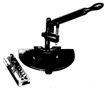
FIGURE IV Punch and extra dies for cutting 1/16 inch lead discs for rifling meter
