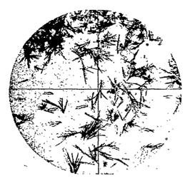
FIGURE 4 Heroin with  $HgI_2$  in 10% HCl. Method B.
