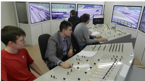
Pic. 2. The operator of the second braking position of the 3 rd and 4 th beam adjusts the speed of rolling of uncouplings depending on weight and the way of classification yard.
