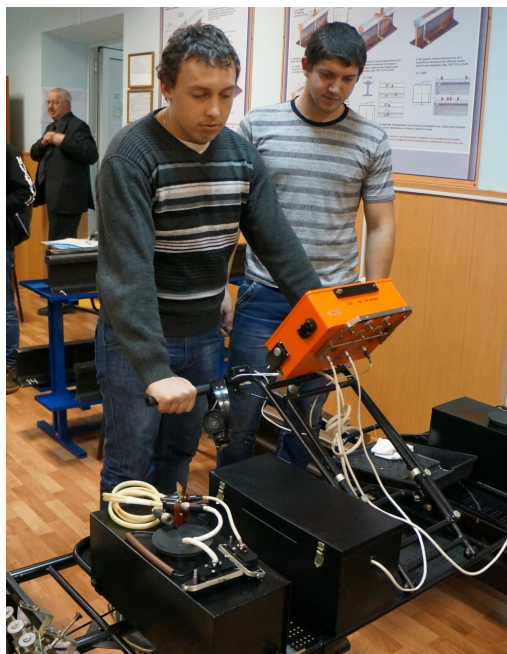
Fig. 5. Identification of defects by double-helical wave detector Avikon-11 at «control dead end».
