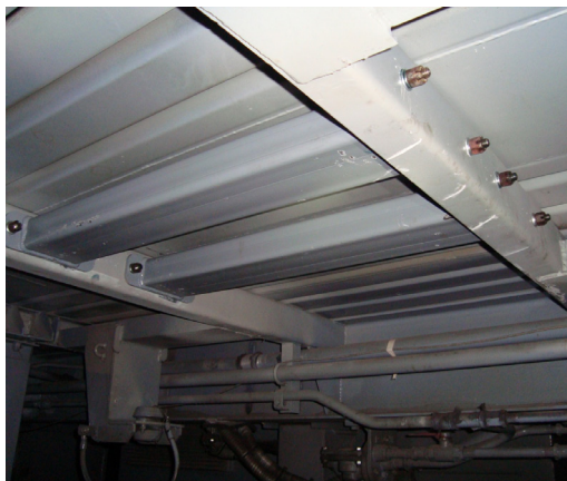
Pic. 2. Frame of the car, reinforced with longitudinal beams.
