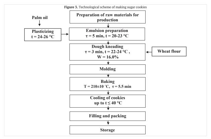
Immediately after making the dough, it was rolled out on an automated rolling machine into a layer 5 mm thick, molded with a metal notch of a round shape, baked on steel sheets and cooled in natural conditions to room temperature.
