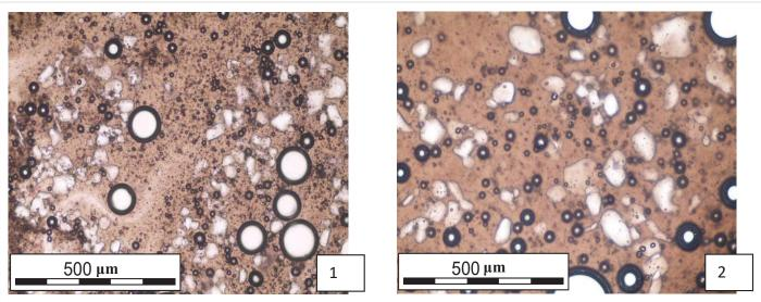
Figure 5. Microphotograph of dispersion of ice crystals of milk ice cream at 4.0% fat content: 1 -after 1 month of storage, 2 -after 8 months of storage
