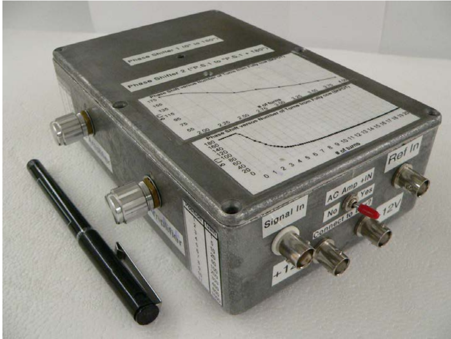
Fig. 2.16: This image is included as a size comparison. The dimensions of our box are 6x4x2 inches. Two holes have been drilled through the top of the box to allow for a screwdriver to fit through in order to change the resistance of the phase shifter potentiometers. The graphs on the box reveal tell us the resistance as a function of the number of turns. The knobs are for the AC and DC gain. Our lock-in amplifier requires a \pm 12V power supply. The input and dither signal channels are also displayed. We also include the option of grounding the input signal to the box.
