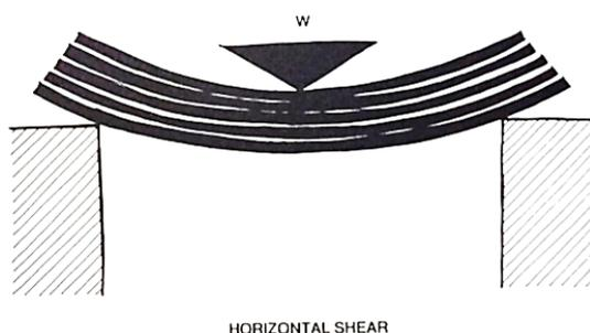
Gambar 7. Horizontal Shear
