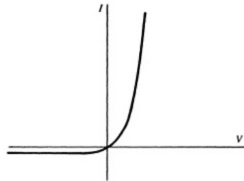
Figure 2: Typical I-V characteristic of a p-n junction.
