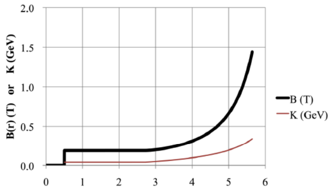
Figure 4: Variation of magnetic flux density, satisfying the isochronous condition (solid line) in the case of simple microtron as a recirculating LINAC. The thin line indicates the kinetic energy K.
