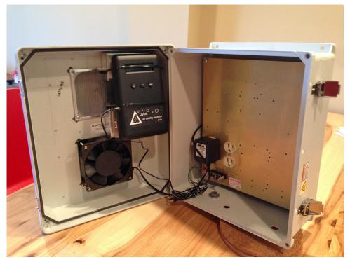
Figure 2. Air monitor system including modified Dylos particle sensor with four size bins (>0.5  $\mu$ m, >1.0  $\mu$ m, >2.5  $\mu$ m and >10  $\mu$ m), temperature and relative humidity sensors, and a microcontroller.
