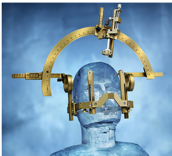
Figure 1. Head frame for stereotactic neurosurgery (courtesy of Elekta®).
