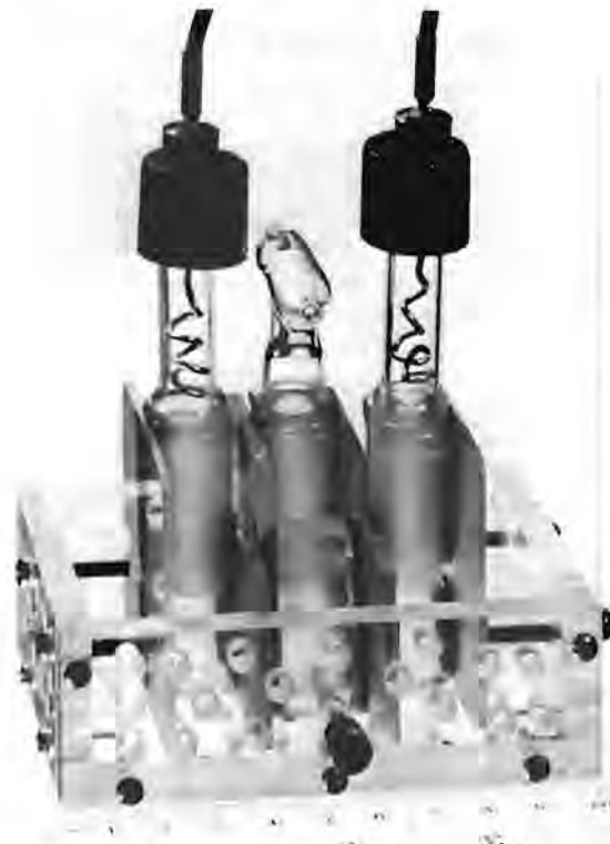
Fig. 4. Electrophoresis device used in attempt to separate bull sperm. (Courtesy of Dr. H. D. Hafs)
