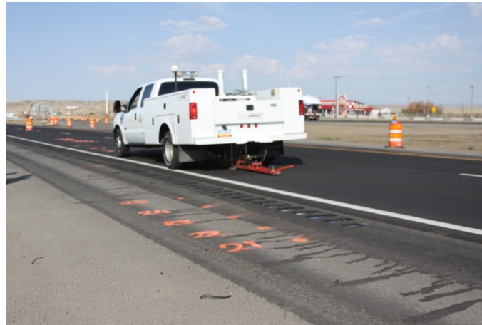
Figure 5. Conduction of FWD test on I-40 pavement.
