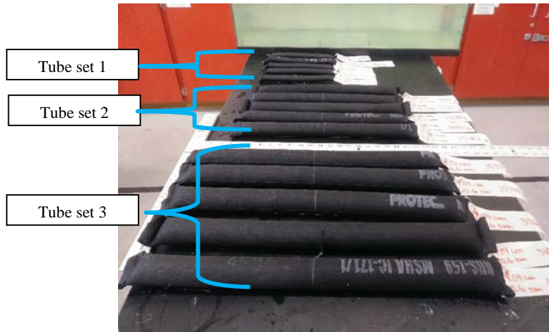
Figure 3. Fully morphed tubes ready for bending test
