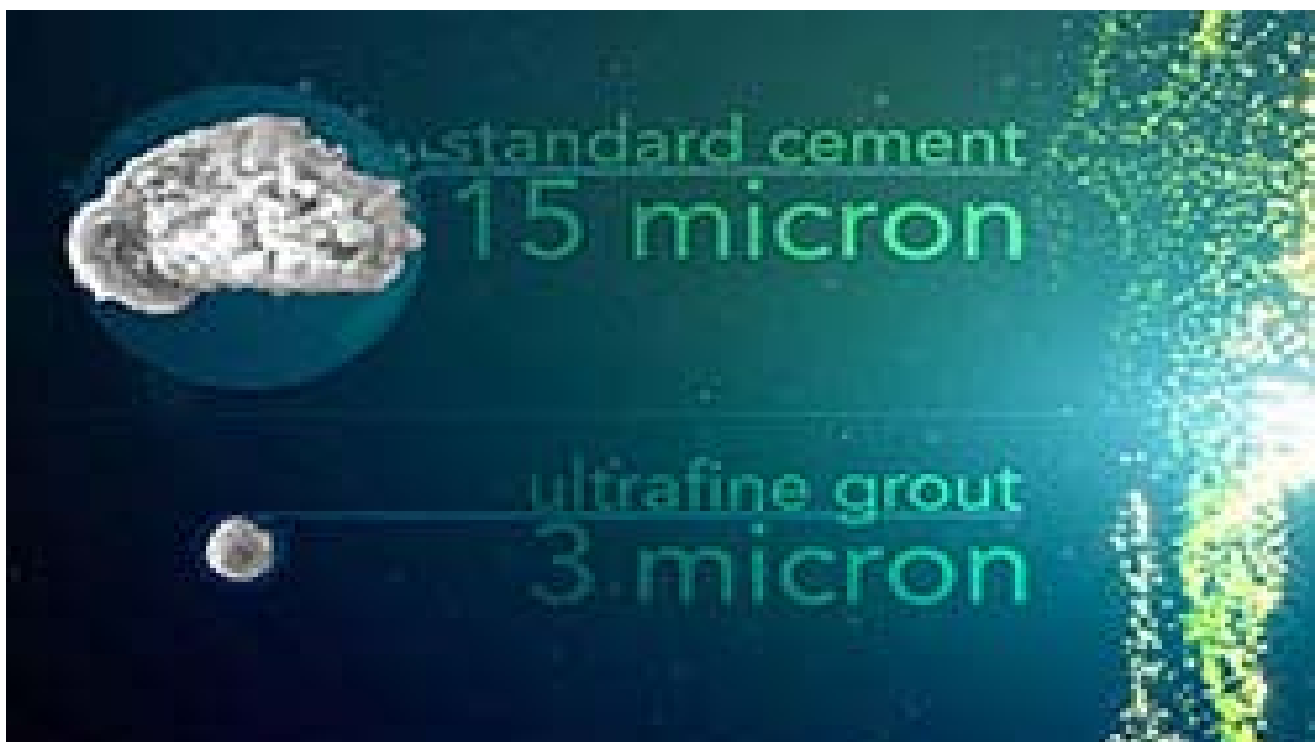
Figure 4. Particle Sizes of Standard cement and ultrafine cement grouts
