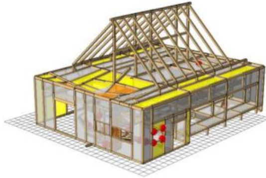
Figure 11. Seismic behaviour after earthquake motion (JR Takatori, With seismic retrofit, Limit strength calculation method 1.5, Unfixed post condition \mu_s=0.3 )
