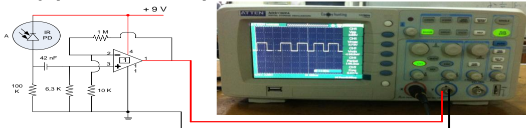
Figure 14 Amplifier testing using high pass filter
