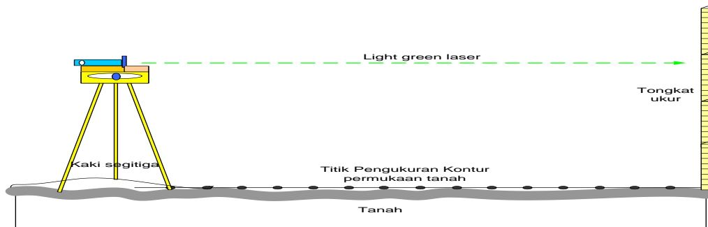
Figure 8 Field measurement and stake position for tractor track
