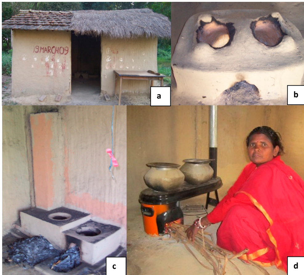
Figure 1. Study I photos of testing house and stoves used in water boiling test study in rural Nepal. (a) Single room test house, (b) traditional stove, (c) alternative mud-brick stove (AMBS-1), and (d) Envirofit G-series stove.
