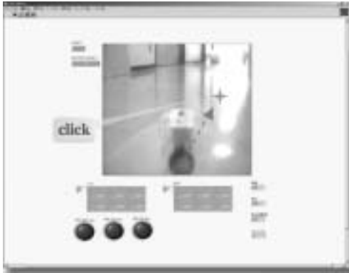
Fig. 2.3.2 The front panel of “Remote navigation VI for a mobile robot (camera-image mouse-click system; robot fixed camera)”. The block diagram of the VI is given in Appendix E.
